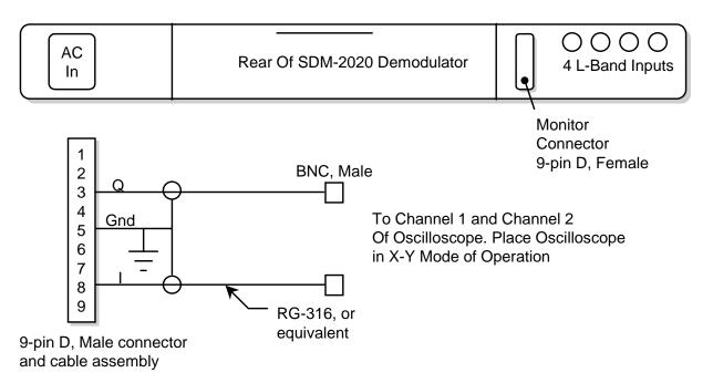
Figure 4 Monitor Connector for Viewing I/Q Constellation on an Oscilloscope
