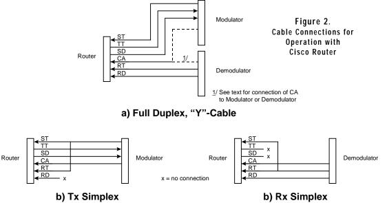
Cisco routers manufactured before September 1998, and possibly later, require special consideration for operation. Since the application note was first released. Cisco has released software updates that should eliminate the need for special wiring of clocks described in this application note. Consult Cisco if there is difficulty with the software updates. As an alternative, try rewiring the cable.
